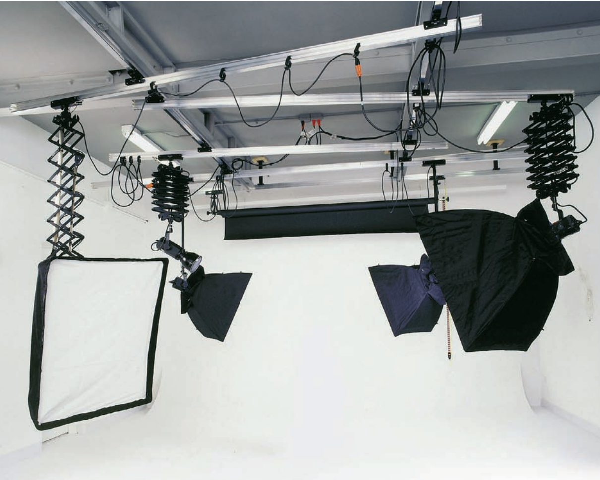
Typical small studio space equipped with high-glide ceiling mounted monoblocs that leave the floor area completely free of clutter.
