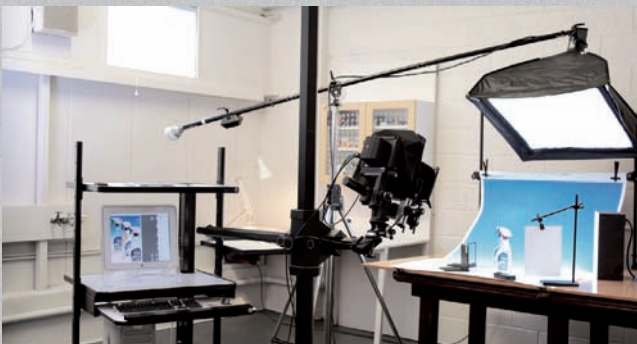
Pack shot studio showing typical arrangement with overhead softbox on boom , graduated colour card background, small strip lights on the tabletop and reflectors. The monorail camera has a digital back controlled by the computer on the table to the left.
